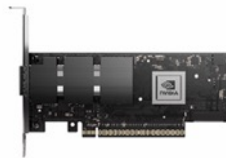
ConnectX-7 400GbE Single-port OSFP, PCIe 5.0 x16
